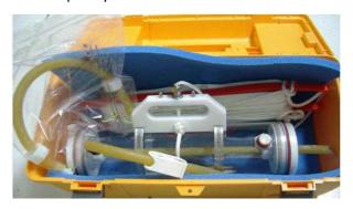
**Notes:** Designed for general limnological use where sampler clarity is important (zooplankton collection, near bottom water recovery w/o contamination, hydrogen sulfide...).
